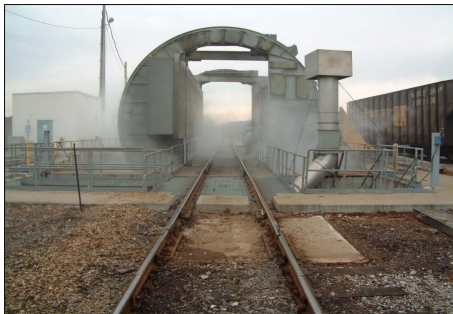
Figure 10: A wagon tippler using dry fog.
