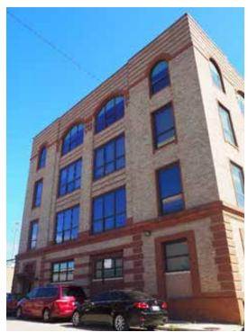
In the Kinzie Industrial Corridor, buildings constructed at the end of the 19th century and early 20th century were frequently constructed of Chicago common brick and accentuated with red face brick details.
