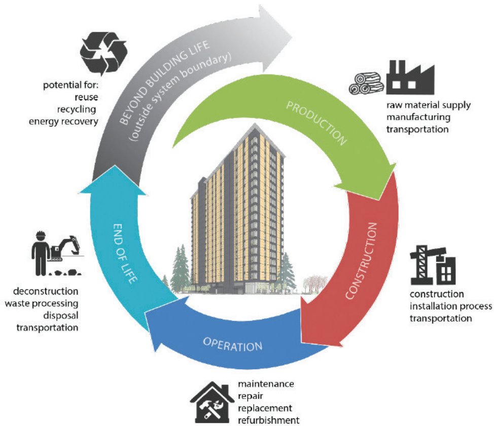
Flow diagram illustrating the building life cycle stages and beyond. Credit: UBC Embodied Carbon Pilot: Study of whole building life cycle assessment processes at the University of British Columbia., 2021
